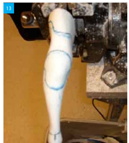
Creation of a custom stifle brace by making a proper cast mold of the affected limb Courtesy Animal Orthocare, animalorthocare.com
